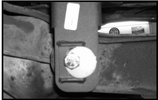
43. The brackets around the "D" bushings on the stock front sway bar may need to be opened up to 7/16". Try a 7/16" bolt in each location to make sure that it will fit. If not, open the holes up so that the new 7/16" bolts will fit.
