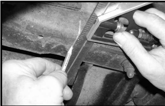
22. Locate the new driver side extended radius arm relocation bracket. Place the line that was scribed on the bottom of the frame rail in the center of the rearward hole that is in the bottom side of the new relocation bracket. Using a pair of vise grips, secure the bracket to the frame rail.
