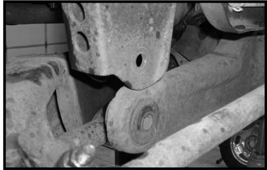
7. Working on the front driver side twin eye beam axle bracket, remove the stock bracket from the stock location. Save the stock hardware but the the stock bracket may be discarded.
