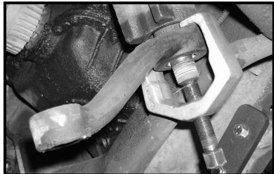
39. Locate the new pitman arm. Locate the stock hardware that connected the stock pitman arm to the sector shaft on the steering box. Install the new pitman arm into the stock location and secure using the stock hardware. Make sure to use thread locker or loctite and torque to **145 ft lbs.**
