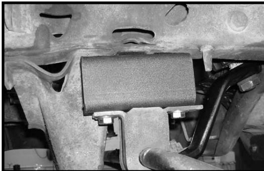
47. Move back to the stock lower sway bar end link mounting hardware and add some thread locker or loctite on both the driver and passenger side and torque to **65 ft lbs.**
