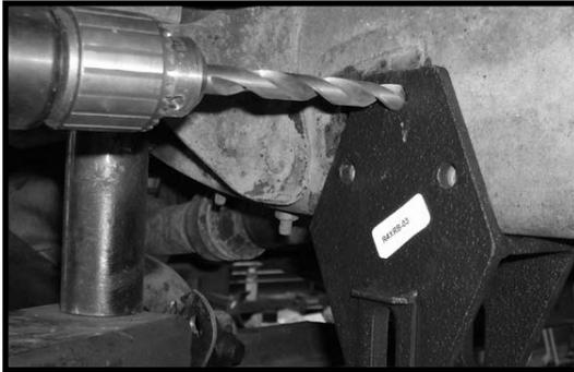
25. Locate (5) 7/16" x 1 1/2" bolts, (10) 3/8" USS flat washers and (5) 7/16" unitorque nuts from hardware bag R4XRB-NB. Secure the driver side extended radius arm to the new location using the new 7/16" x 1 1/2" bolts and hardware. Make sure to use thread locker or loctite and torque to **45 ft lbs.** **Special note: Make sure to secure the stock brake cable bracket to the front hole that connects the bracket to the side of the frame rail.**
