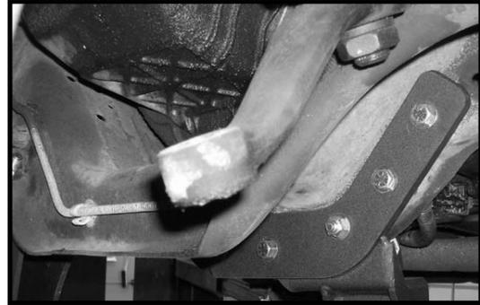
38. Remove the stock hardware that connects the stock pitman arm to the sector shaft on the stock steering box. Save the hardware. Using a pitman arm puller, carefully remove the pitman arm from the stock location. The pitman arm may be discarded.
