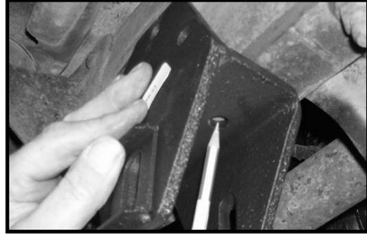
23. Using the bracket as a guide, carefully outline each hole of the bracket onto the frame rail. There are (3) on the side of the frame rail and (2) on the bottom side of the frame rail. Remove the bracket from the frame rail and set the bracket a side.
