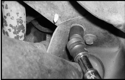
10. Locate the new front twin eye beam relocation bracket and the stock hardware. Install the new front relocation bracket to the stock location and secure using the stock hardware. Make sure to use thread locker or loctite and torque to **85 ft lbs.**
