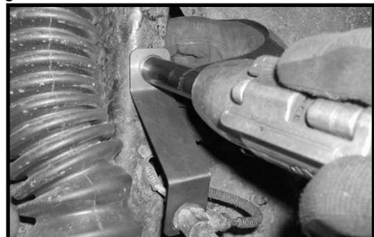
52. Locate (2) e-clips from hardware bag FBLNB2. Working on the driver side, install the new e-clips to the stock brake line on the back side of the newly installed brake line relocation bracket. Repeat procedure on the passenger side. **Special note: Once the installation of this suspension is completed and the weight of the vehicle is on the ground, check to make sure that the stock brake line does not rub on the inside of the tire.**
