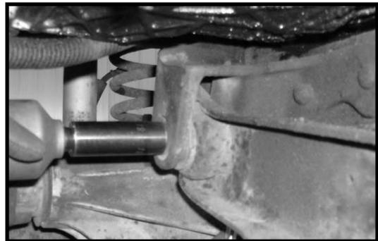
9. Working on the driver side stock radius arm bracket, remove the stock hardware or the stock rivets that connect the bracket to the frame rail. The stock hardware and rivets may be discard. Repeat procedure on the passenger side. **Special note: Using a die grinder and making a cross cut on the rivets then using a air chisel will help make the removal of the rivets easier.**
