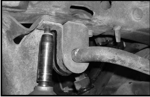
4. Working on the driver side, remove the stock sway bar end link from the stock axle location. Save the hardware. Repeat procedure on the passenger side. Set the sway bar aside.
