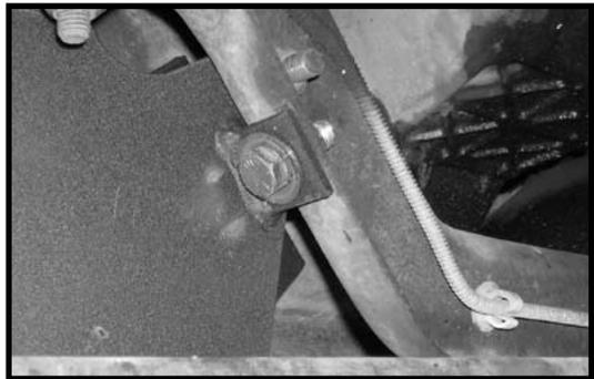
13. Working on the stock rear axle pivot relocation bracket, remove the rivets holding the bracket to the cross member. **Special note: Using a die grinder and making a cross cut on the rivets then using a air chisel will help make the removal of the rivets easier.** The stock bracket may be discarded. Carefully drill out the (5) rivet holes to 7/16".
