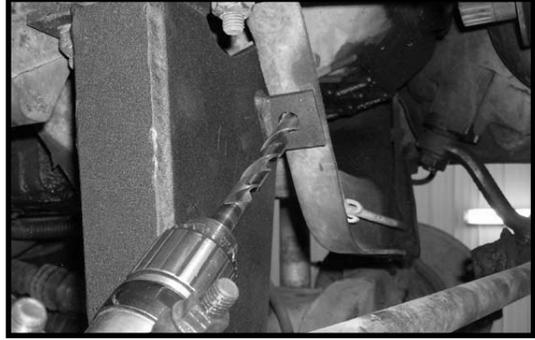
12. Locate (1) 1/2" x 1 1/2" bolts, (2) 7/16" USS flat washers and (1) 1/2" unitorque nuts from hardware bag R4NB. Secure the newly installed front axle pivot relocation bracket to the front cross ember using the new 1/2" x 1 1/2" bolt and hardware. Make sure to use thread locker or loctite and torque to **75 ft lbs.**
