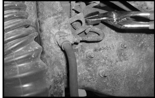
50. Locate the new front brake line relocation brackets from hardware bag FBLNB2. Working on the driver side, slide the open end of the new brake line over the stock brake line. Now measuring from the stock brake line hole up 2 1/2", carefully drill a 5/16" hole into the stock shock/coil spring bucket. Repeat procedure on the passenger side. **Special note: Take special care not to damage the stock brake line when performing this step.**
