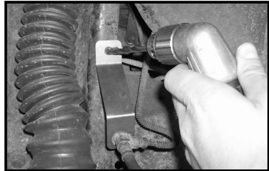
51. Locate (2) 5/16" x 1" bolt, (4) 1/4" USS flat washers and (2) 5/16" unitorque nuts from hardware bag FBLNB2. Working on the driver side, secure the new front brake line relocation the to the previously drilled hole using the new 5/16" x 1" bolt and hardware. Make sure to use thread locker or loctite and torque to **12 ft lbs.** Repeat procedure on the passenger side.
