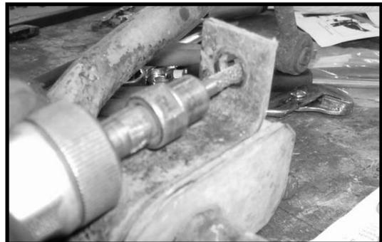
44. Locate the stock sway bar and the stock sway bar lower hardware. Working on the driver side, install the stock sway bar end link into the stock lower location and secure using the stock hardware. **Do not tighten at this point.** Repeat procedure on the passenger side. Let the stock sway bar hang.
