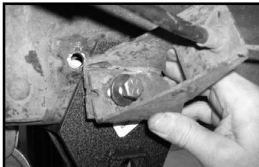
26. On the passenger side where the new extended radius arm bracket will be located there is a lip on the bottom of the frame rail. This lip needs to be removed so that the extended radius arm relocation bracket will sit flush on the frame rail. Carefully cut lip off with a die grinder. **Special note: Tuff Country does not recommend using a torch when performing this step.**
