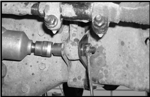
5. Place a pair of hydraulic floor jacks under the front driver and passenger side twin eye beam axles. Carefully raise up on the hydraulic floor jacks until they come into contact with the front twin eye beam axles. Also, place a pair of hydraulic floor jacks under the driver and passenger side stock radius arms. Carefully raise up on the hydraulic floor jacks until they come into contact with the stock radius arms.
