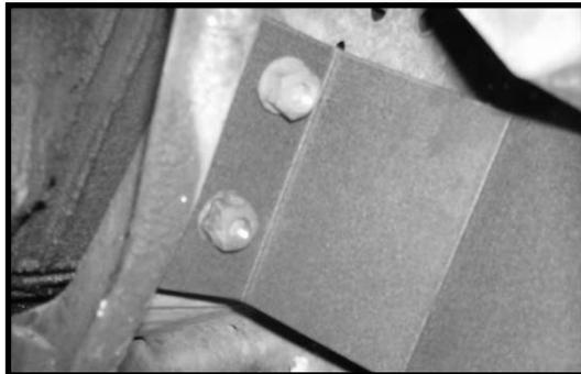
11. Working on the newly installed front twin eye beam axle pivot relocation bracket and using the tab on the bracket as a guide, carefully drill a 1/2" hole into the stock front cross member. **Special note: Take special care not to drill into the cooling lines that wrap around the front cross member. Also, drilling a pilot hole first may make drilling easier.**
