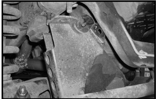
8. Working on the rear passenger side twin eye beam axle, remove the stock mounting hardware that connects the rear axle to the stock location. The stock hardware may be discarded.
